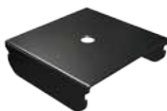
Single spaced hanger 5 mm Ø 6 MA for C Plus profiles 50/15 · 50/27 · 60/25 th. 1.2 mm for ceilings and wall linings
